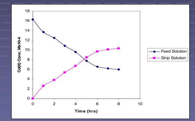
Decrease in concentration of Cd(II) ions in feed vs. time for aqueous effluent. [NaOH]=0.5M, [TEA]=3.0M, [HCI]=2.0M, [Cd(II)]=33ppm
